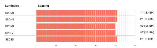
Average spacing for 1 out of every 4 luminaires, normally ON in the path of egress, when at 8, 10, or 12 foot mounting heights.
