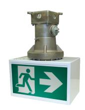
The RPHZ series of hazardous location running man signs are designed to meet and exceed the most stringent code requirements. The housings are made from copper free, heavy-duty die cast aluminum. The frame and faceplate(s) are manufactured in heavy gauge steel with a white, powder coating finish. The signs can be specified to suit a variety of mounting options including ceiling, wall and pendant mount.
